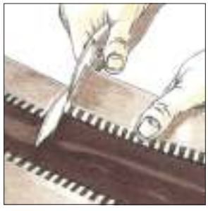
At a notch, cut a length equivalent to the perimeter required plus an overlap of 5 to 6 cm (2") for joining
