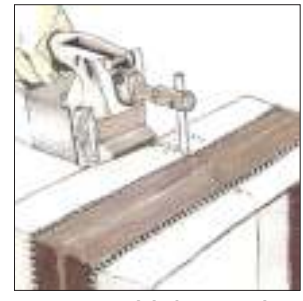
Spotweld the steel and form to the desired shape
