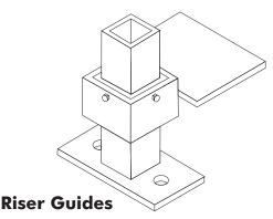
Capacities from 650 lbs. and up, for vertical and horizontal load applications.
